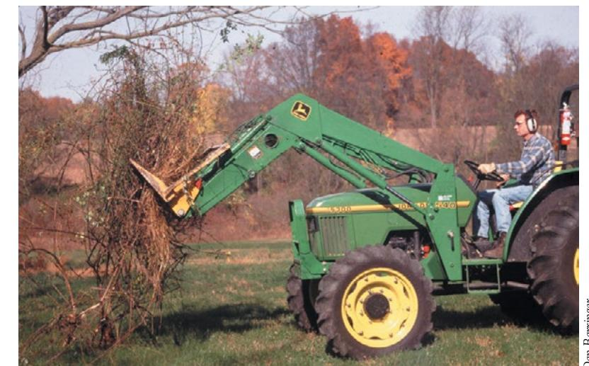
An efficient method for removing unwanted shrubs or small trees involves replacing the loader bucket on a tractor with a Brush Brute to impale the base of the plant and then lift it out of the ground. When using this method, care must be taken to minimize soil disturbance.
